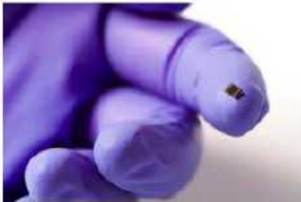
World record solar cell with 44.7% efficiency, made up of four solar subcells based on III-V compound semiconductors for use in concentrator photovoltaics. ©Fraunhofer ISE
